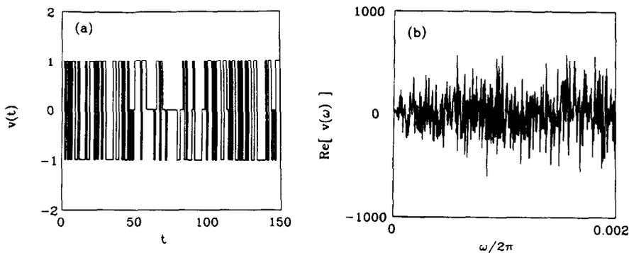
Fig. 1. One-dimensional particle diffusion with hard-core interaction (at particle density 1/4). (a) The typical velocity plot of one particle. The velocity was recorded for a very long time period ( $2^{14}$  time steps), only part of them are shown here. (b) The Fourier spectrum for the same particle.
