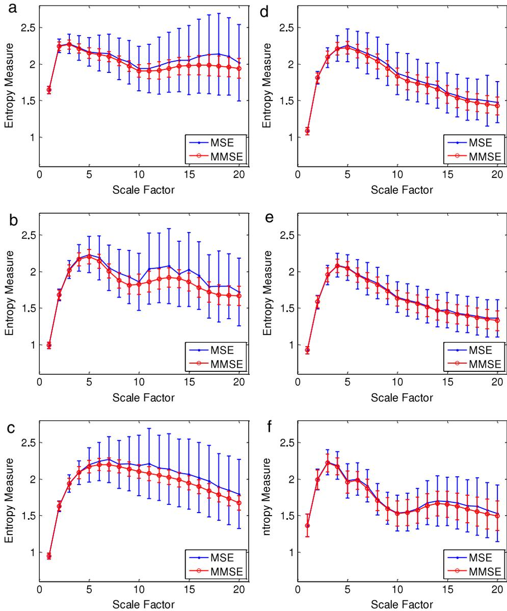
**Fig. 6.** MSE and MMSE results of bearing vibration data (1730 rpm, 7 mils): (a) normal state; (b) ball fault; (c) inner race fault; (d) outer race fault (3 o'clock position); (e) outer race fault (6 o'clock position); and (f) outer race fault (12 o'clock position).
