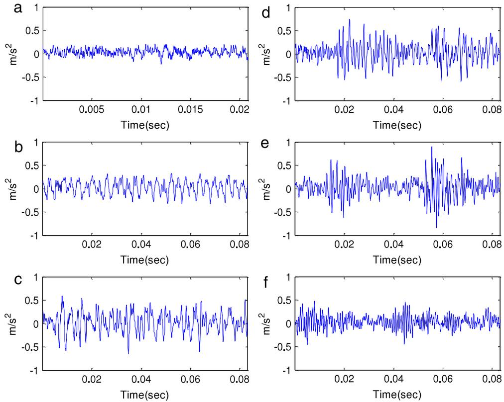
**Fig. 5.** Bearing vibration data in the time domain (1730 rpm, 7 mils): (a) normal state; (b) ball fault; (c) inner race fault; (d) outer race fault (3 o'clock position); (e) outer race fault (6 o'clock position); (f) outer race fault (12 o'clock position).
